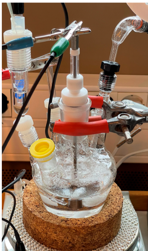
Figure 4. Experimental setup for CO 2 corrosion inhibition testing.
