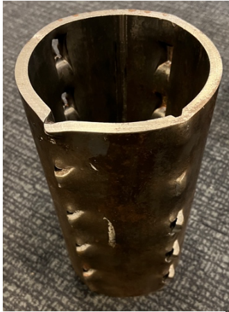
Figure 23 – Casing after Slot Jet Isolate [23]
