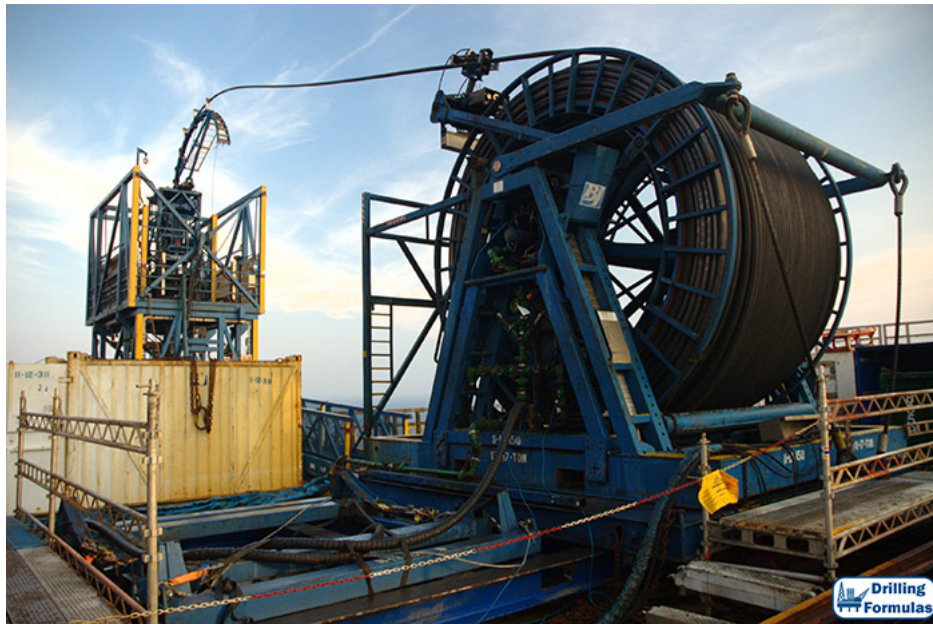
Figure 8 – Coiled tubing reel and injector with gooseneck [18]
