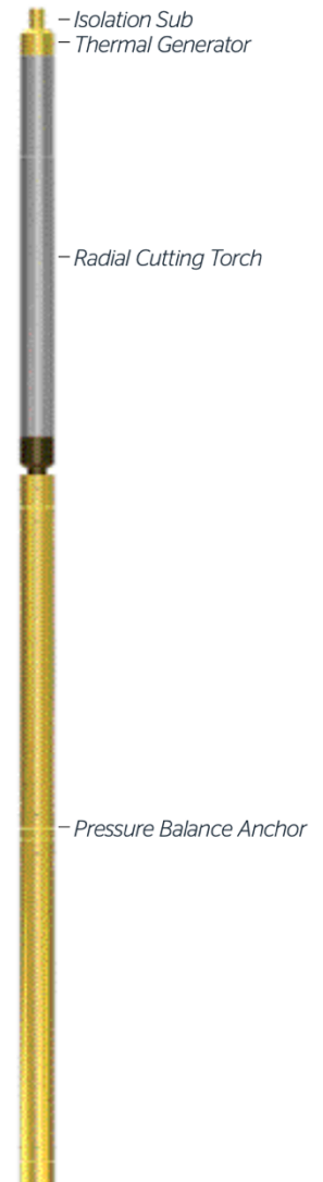
Figure 16 – Components of the Radial Cutting Tool [30]
