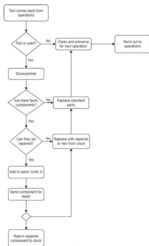
Figure 3. Process flowchart for the enhanced scenario with repair path [8]
