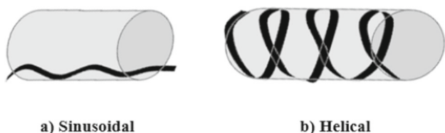
Fig. 9 Three-dimensional schematic of sinusoidal and helical buckling [37]
