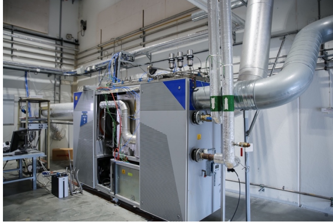
Figure 3.8 Turbec T100 unit with modified combustor and fuel train for flexible fuel operation.
