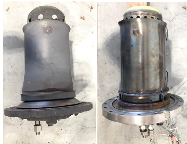
Figure 5. The original combustor was installed on T100 (left) compared to the F400s fuel flexible combustor installed on the test rig (right).
