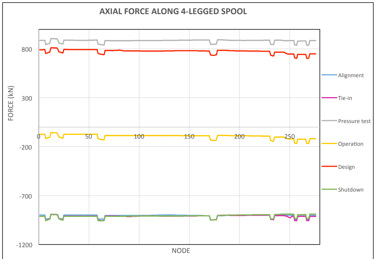
Figure 45: Axial force along 4-legged spool
