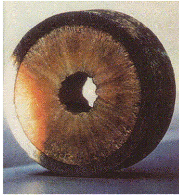
Figure 1.02 Paraffin depositional problems [12].
