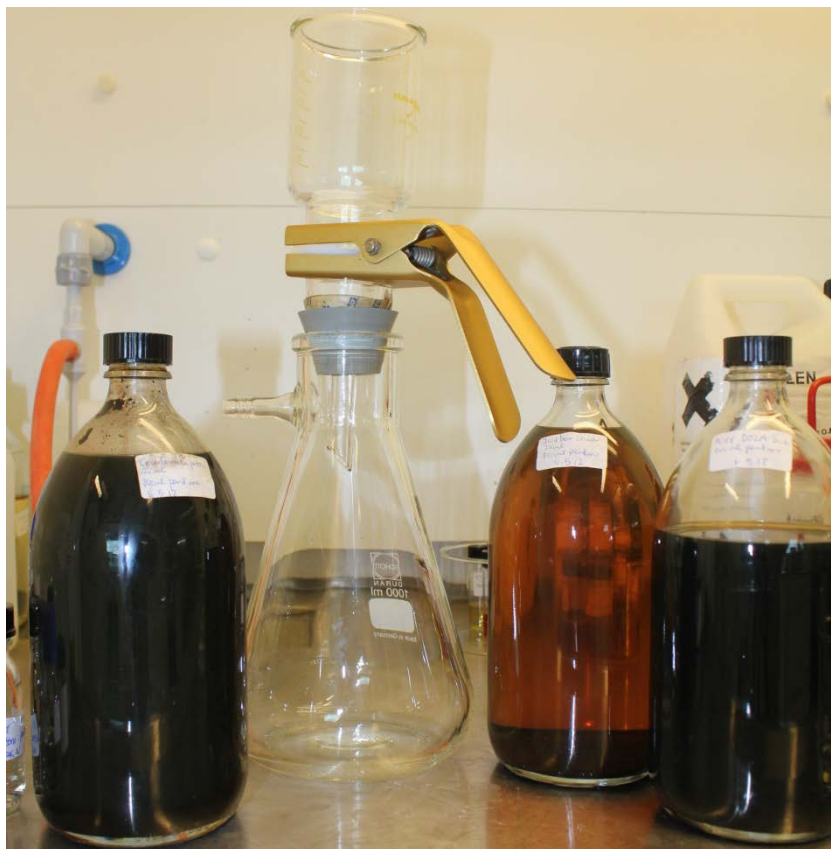
Figure 8.01 The filter assembly and the three flasks of crude oil mixture. From left to right: Crudo-Metapetroleum mixture, Jordbær mixture and Hier D02A mixture.
