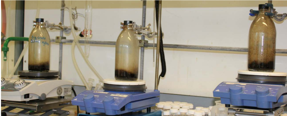
Figure 6.01 Titration layout, bottles with the samples (from left to right) 10ml xylene, 15ml xylene and 20 ml xylene samples placed on the magnet stirrer.
