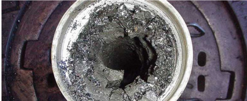
Figure 1.01 Asphaltene depositions in a pipe ( http://www.bakerhughes.com 25.04.12)
