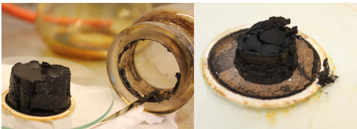
Figure 8.05 (Left) Crudo-Metapetroleum deposit "cake" right after the filtration ended. (Right) The second half of the dried Crudo-Metapetroleum asphaltene deposit.
