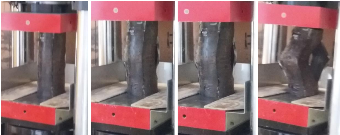
Fig. 5-10 pipe collapse stages
