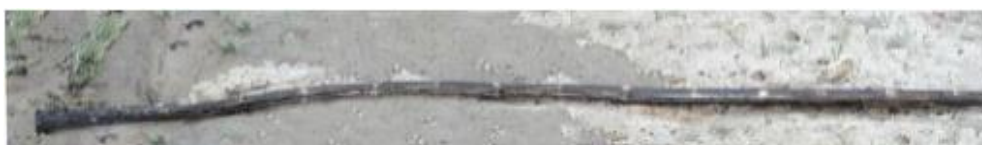
Fig. 3-25 Run 1- plastic buckling deformation [17]
