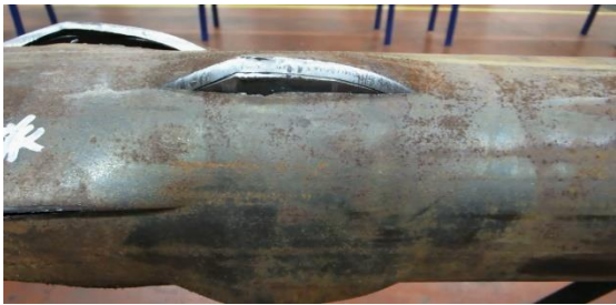
Fig. 3-8 Premature Deformation after perforating by Gator perforator (Lee Energy)
