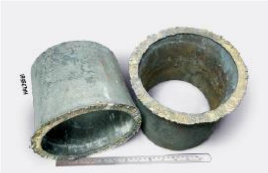
Fig. 2-7 tubing cross section after using explosive cutter [10]
