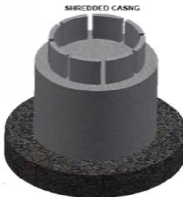
Fig. 3-36 longitudinally slicing casing solution [19]
