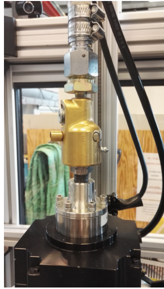
Figure 2.1: Picture showing the connection between the hose, swivel and motor [6].
