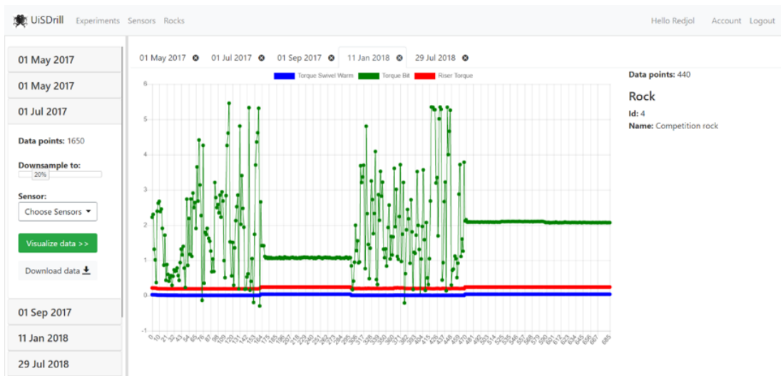
Figure 3.2: Illustration of how data is visualized after the user has selected which sensors and sample resolution to capture. The data can then be exported as a CSV-file.
