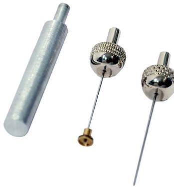
FIGURE 3.6: Vicat test needles
