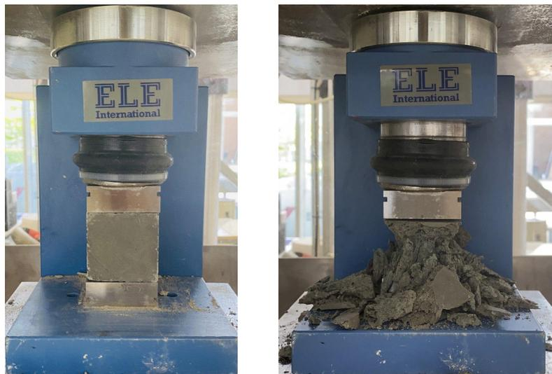
FIGURE 4.5: A cubic specimen collapsed under applied load.
