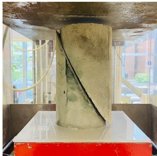
FIGURE 4.6: A collapsed slant shear specimen
