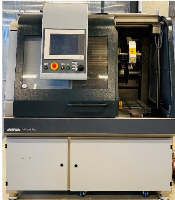
FIGURE 4.2: Cutting machine ATM Brilliant 285
