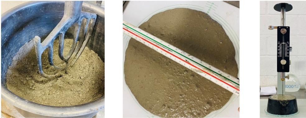
FIGURE 4.4: Blending dry material and immediately after tests
