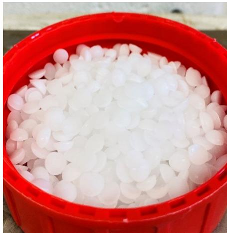
FIGURE 3.2: The potassium hydroxide in solid phase.
