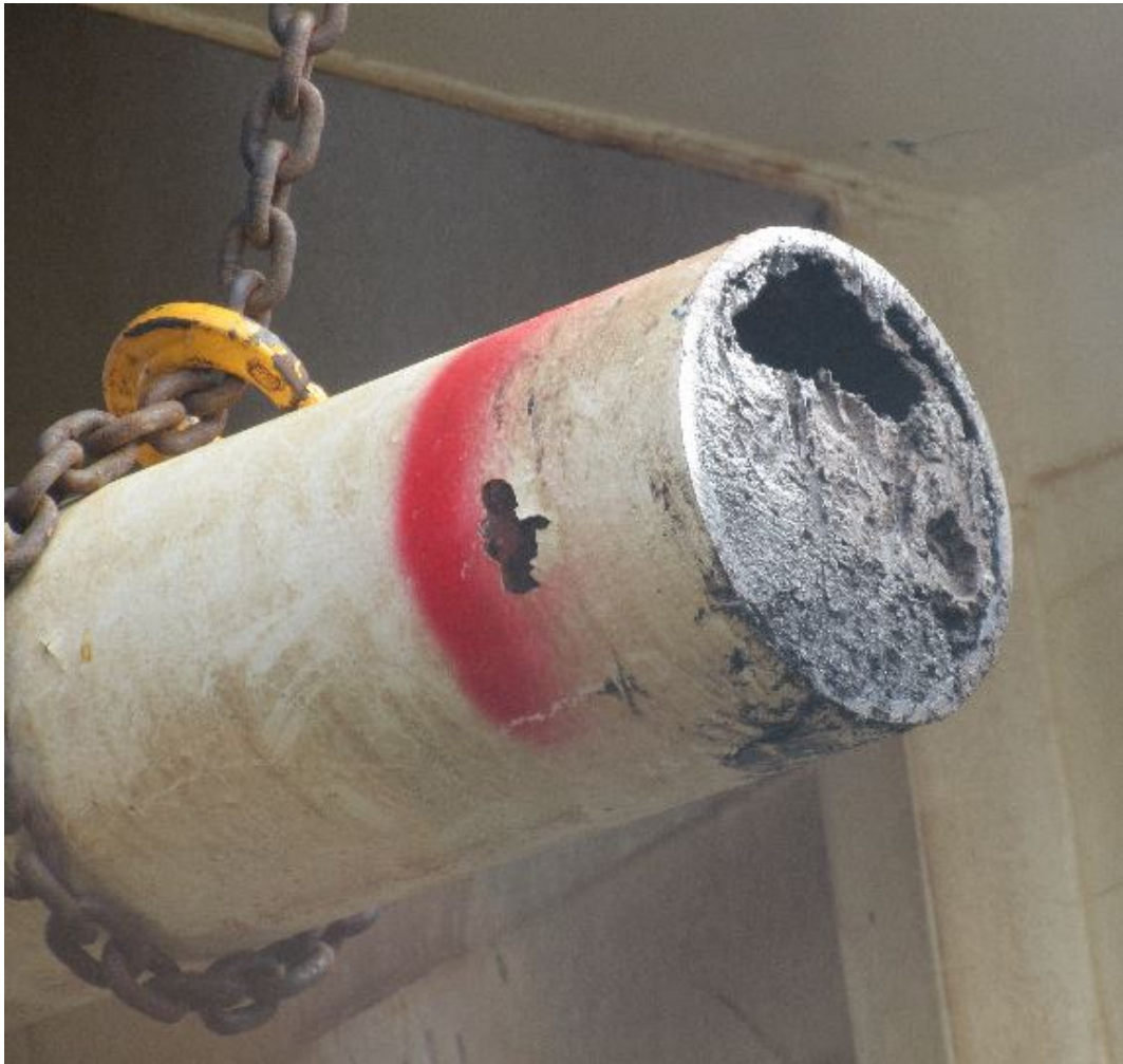
Figure 5.10: Plugged pipe with settled barite due to circulating settled barite out of a well (Equinor 2020)
