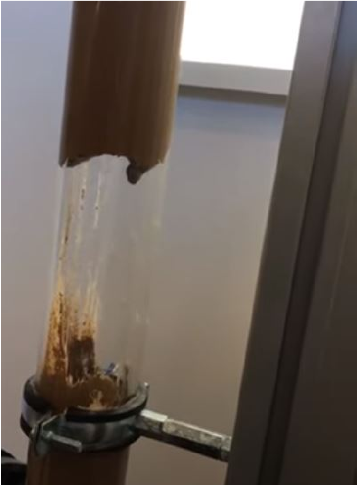
Figure 3.6: Settled micronized barite acts as a plug when pressurized from below with gas (Khalifeh 2021)
