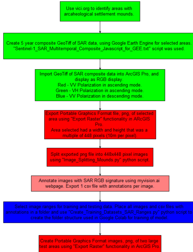
Figure 4.4: Process for generating training and testing data for faster R-CNN model training in Google Colab.
