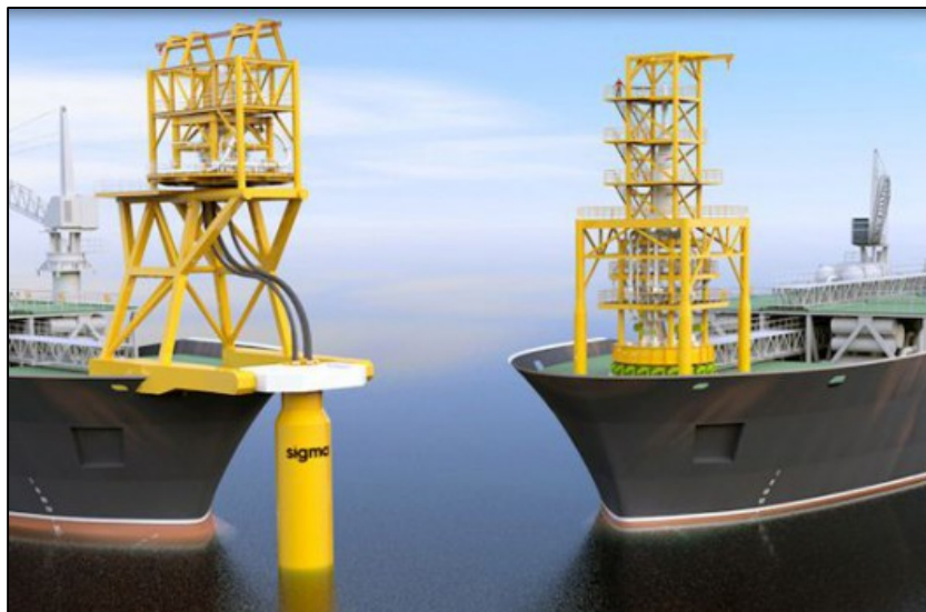
Figure 30: External turret vs. internal turret (47)
