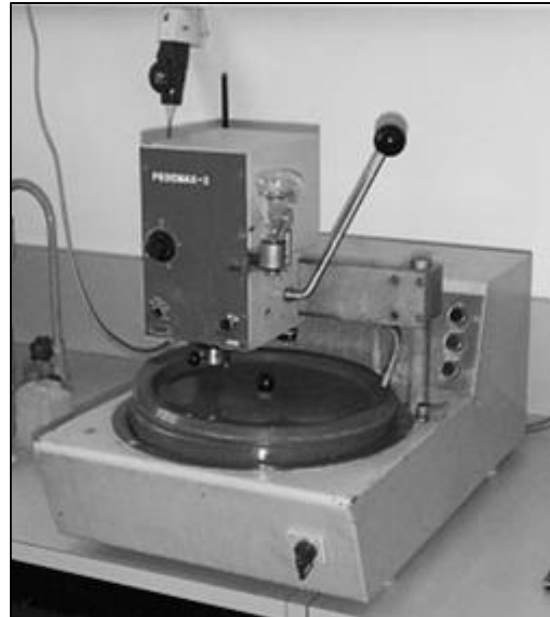
Struers Planopol pedemax-2 automatic grinder and polishing machine. Used to prepare samples for metallographic examination
