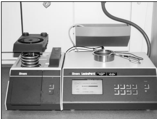
Struers lectropol-5 apparatus for electrolytical etching of metallographic specimens
