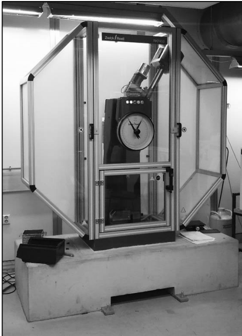
Zwick-Roell RKP450 Charpy V-notch Impact test machine 450J capacity
