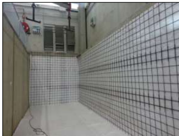
Figure 56: The tank inner surface covered with material and grid plates on top of it
