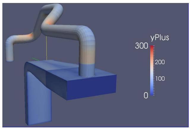
Figure 23: yPlus value for top entry case with refined mesh
