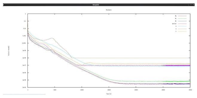
Figure 24: Example of oscillating residuals
