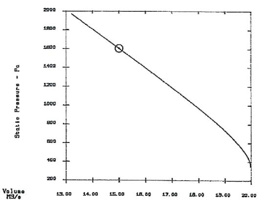
Figure 1: fan performance curve
