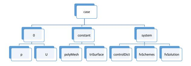
Figure 3: case structure OpenFOAM
