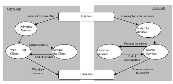
Figure-4: State diagram for server-side and client-side activities
