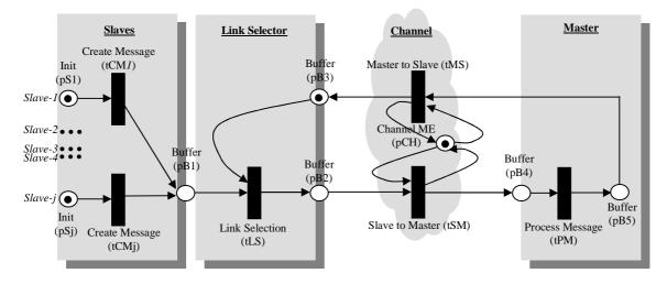
Figure-7: Petri net model of the Piconet-based Assignment Test
