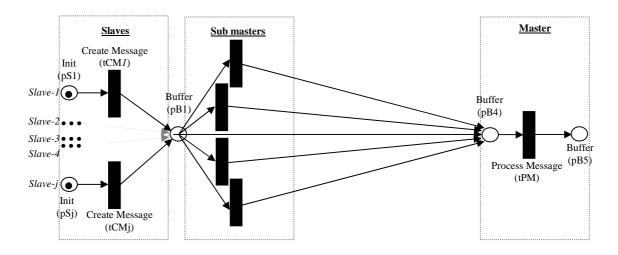
Figure-9: Petri net model of the Scatternet-based Assignment Test
