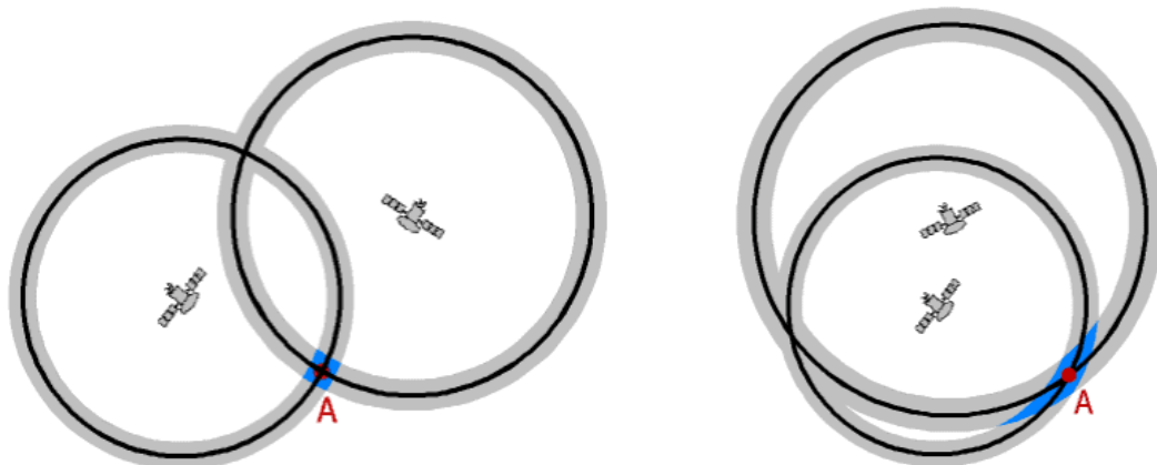
Fig. 7.1: Good versus bad satellite geometry [20]. The good on the left.
