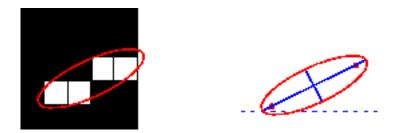
Figure 10: Axes and orientation of the ellipse [3].
