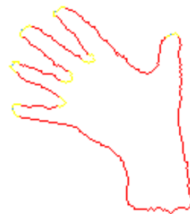
(b) Hand contour with curve points and fingertip location.
