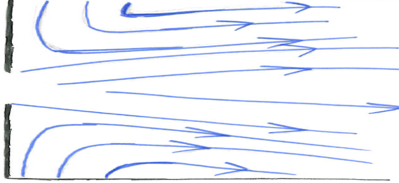
Figure 2.3: Illustration of how we would expect the stream function of a cylindrical jet to behave. We note how the surrounding fluid is being entrained onto the jet .
