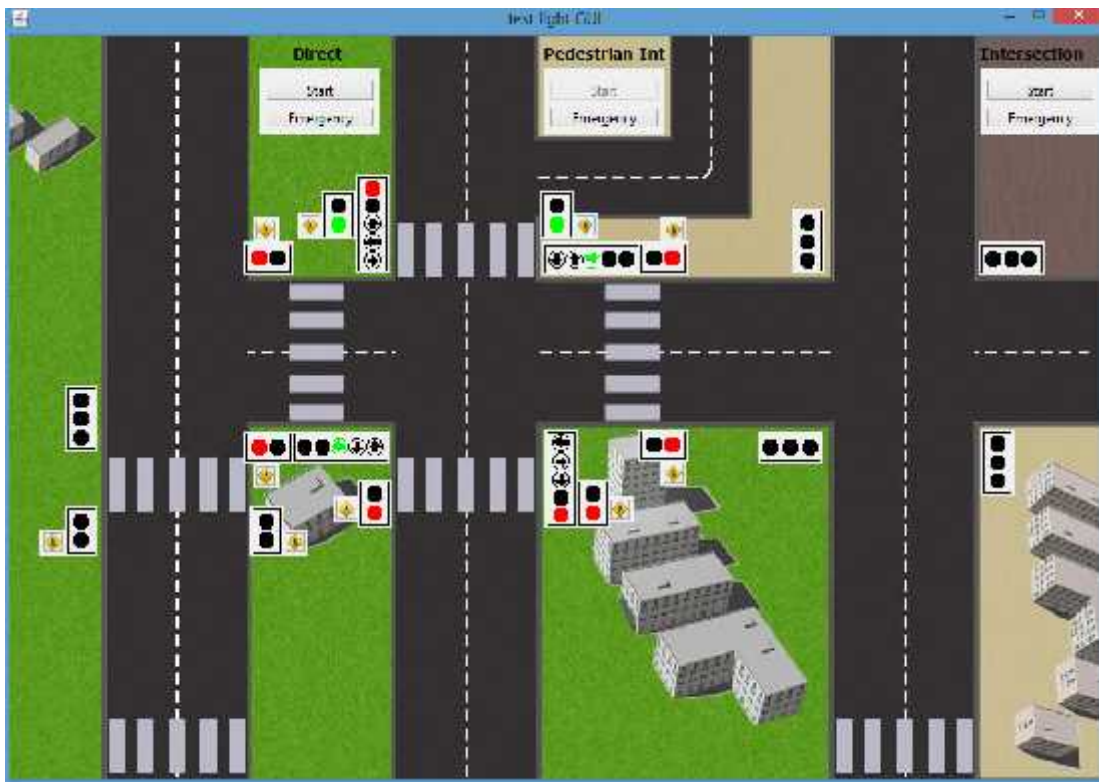
Figure 19: Pedestrian cycle in the North direction for complex intersection
