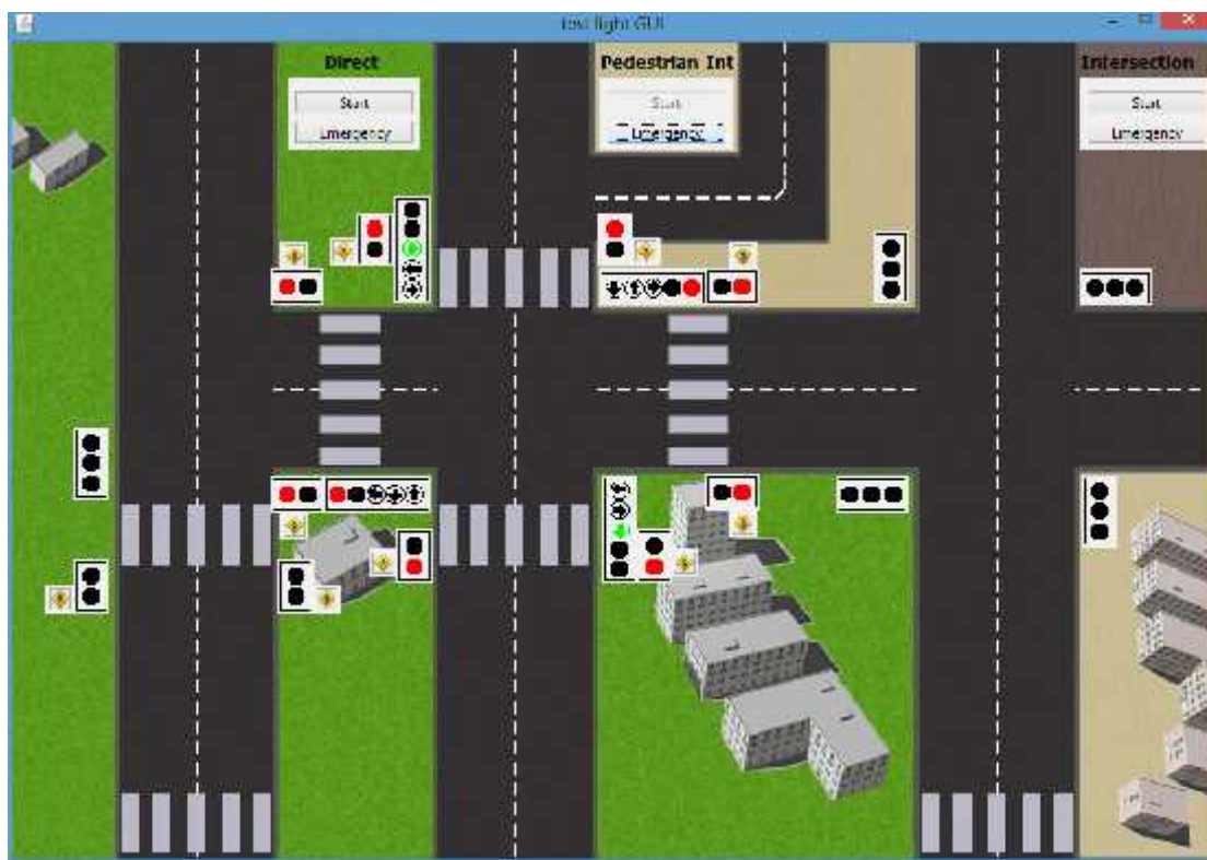
Figure 17: Normal cycle for complex intersection
