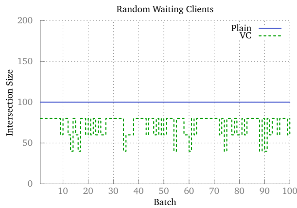
Figure 6.18: A workload where the client waits a random amount of time between sending each request. In this case, there were 20 clients sending 2000 commands. Each client sends a request, and then waits a random period of time between 0 – 20ms before sending the next. This figure shows the first 100 batches.
