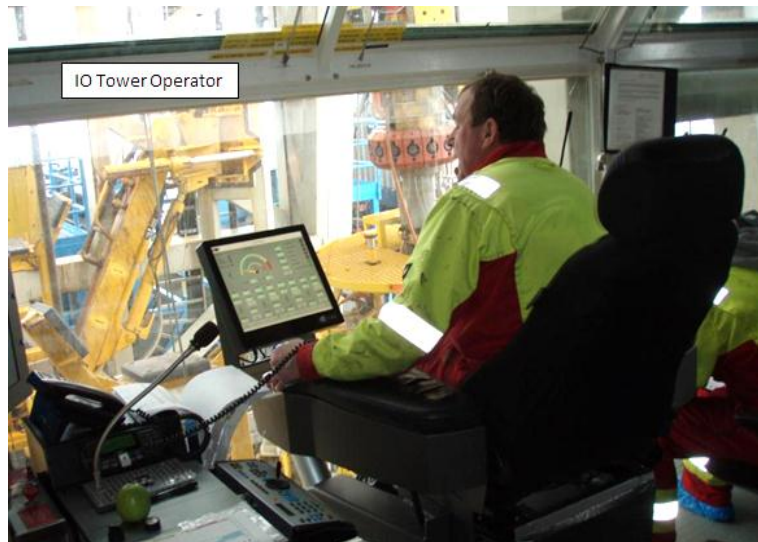
Figure 21: The tower operator panels and seats. The picture is taken at the Island Constructor vessel to be used in this thesis.
