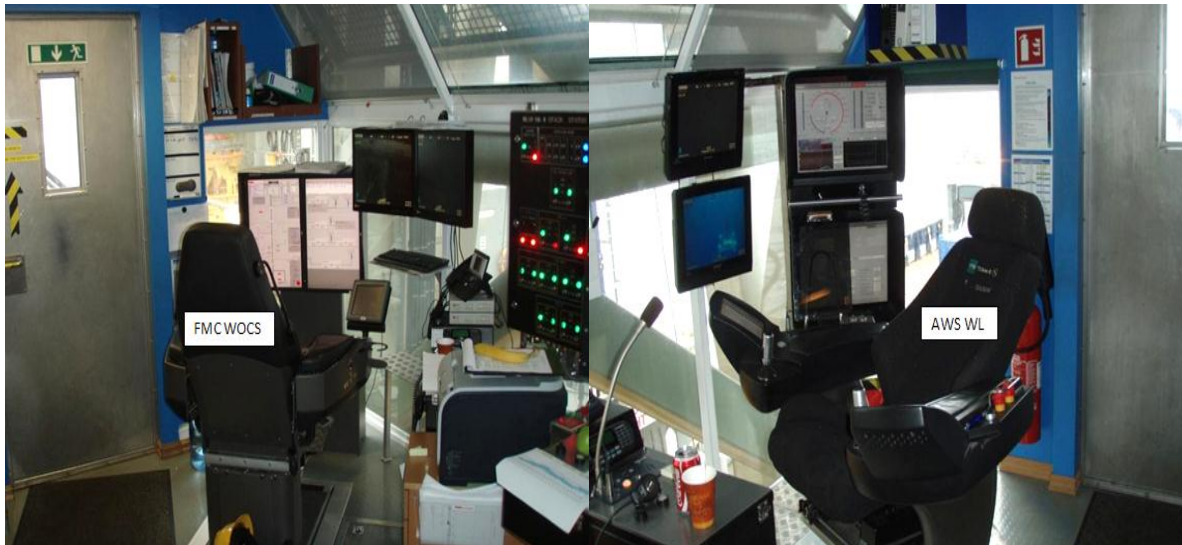
Figure 20: The WOCS and wireline operator's panels and seats. The pictures are taken at the Island Constructor vessel to be used in this thesis.
