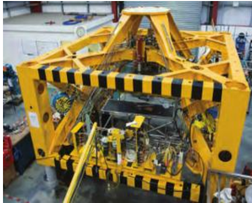
Figure 10: The Running Tool (AX-S, 2011).
