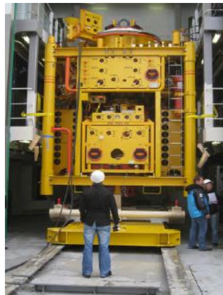
Figure 8: Well Control Package (Island offshore, 2009).
