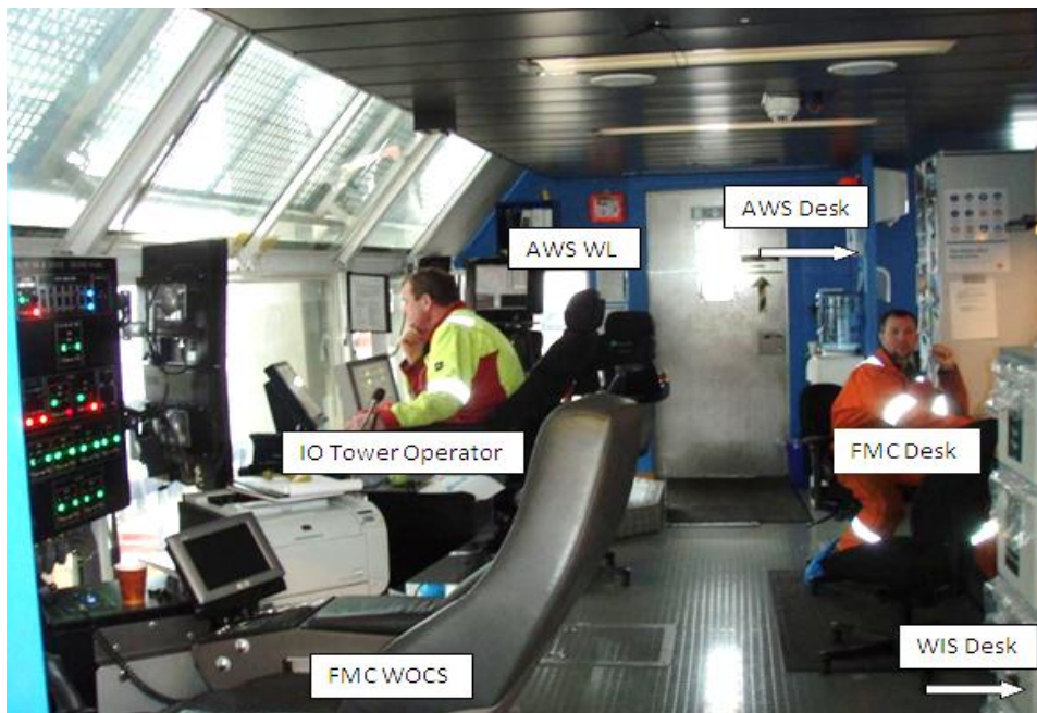
Figure 19: The Tower Control where RLWI operations are performed. The picture was taken at the Island Constructor vessel to be used in this thesis.
