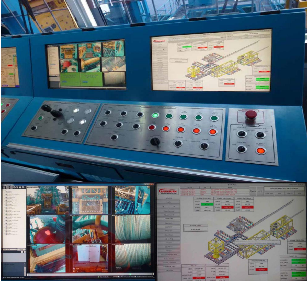
Figure 26: The control system layout in the Deployment Cabin presented at the screens. The pictures were received from Expro to be used in this thesis.
