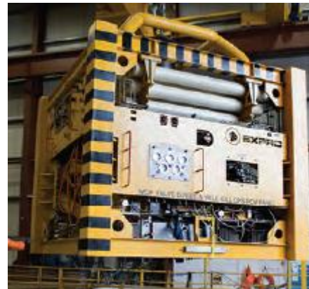
Figure 14: The Well Control Package (AX-S, 2011).
