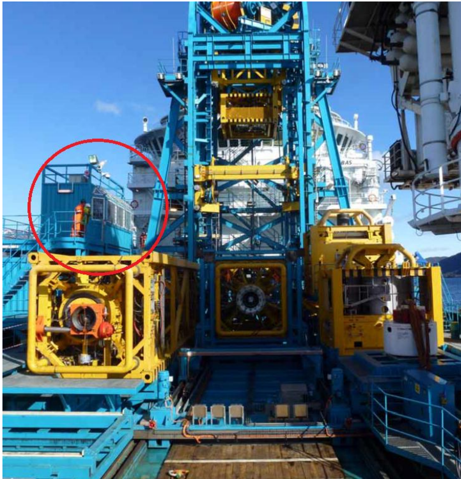
Figure 23: The location of the Deployment Cabin. The Intervention Cabin is placed straight under this cabin. The picture was received from Expro to be used in this thesis.
