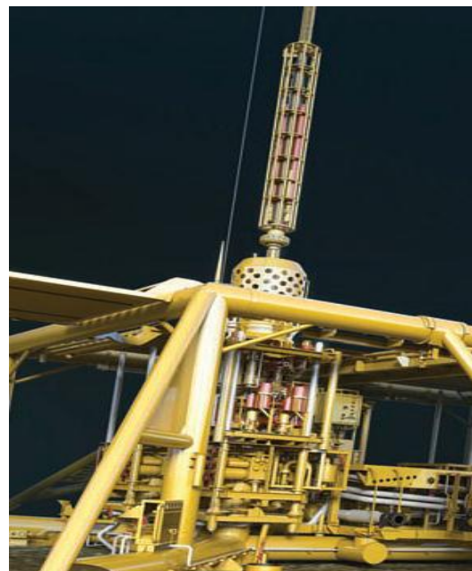
Figure 6: The subsea Lubricator, the Lower Lubricator Connector and the Well Control Package (FMC Technologies, 2008)
