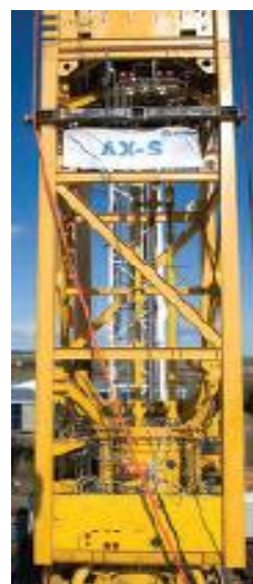
Figure 12: The Wireline Winch Package (AX-S, 2011).
