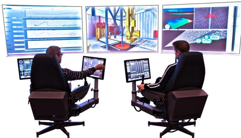
Figure 24: Driller and assistant driller's view over parameters during drilling.
