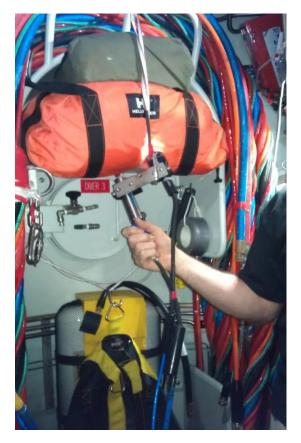
Figure 4: Diver's seat inside diving bell with back-up air supply (Walters, 2012)
