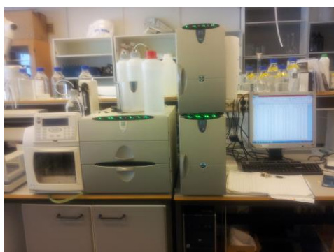
Figure 3.2: Dionex ICS-3000 Ion Chromatograph.
