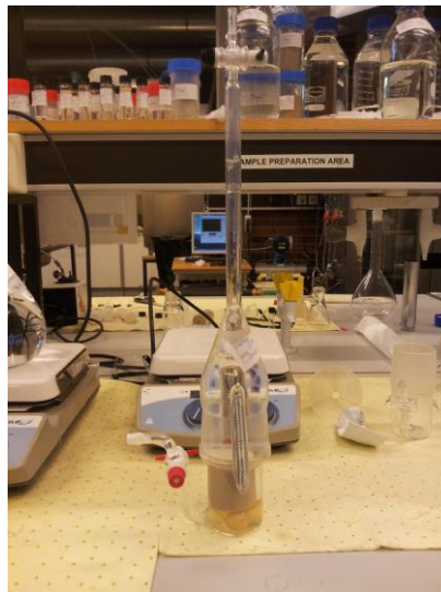
Figure 3.3: Amott cell used for imbibition experiments.
