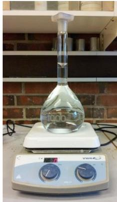
Figure 4-3: Stirring the solutions in a conical flask with a magnetic bar.
