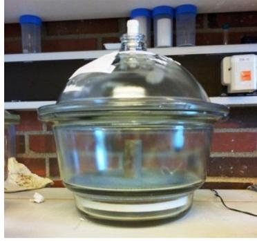
Figure 4-10: Desiccator with Yme Core#22 and silica gel.
