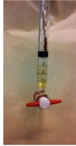
Figure 4-12: Burette with effluent water and oil.
