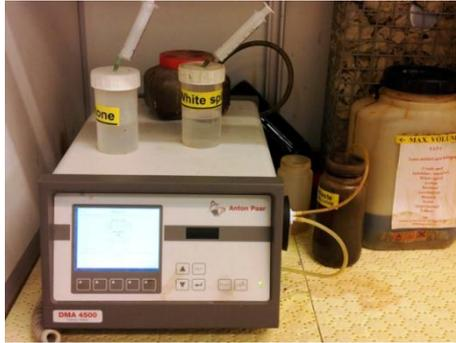
Figure 4-8: A DMA 4500 Anton Paar Density Meter.
