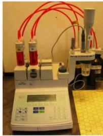
Figure 4-5: The titrating apparatus for measuring AN and BN (Melberg, 2010).
