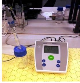
Figure 4-13: METTLER TOLEDO pH meter.
