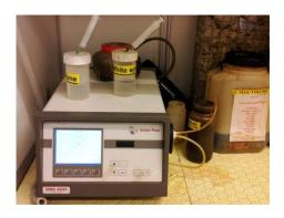
Figure 4-8: A DMA 4500 Anton Paar Density Meter.
