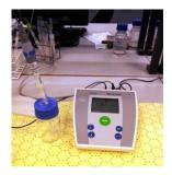
Figure 4-13: METTLER TOLEDO pH meter.
