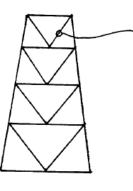
If this element is destroyed, for instance by collison with a vessel, the other elements must be able to withstand the defined loads without suffering a severe collapse
