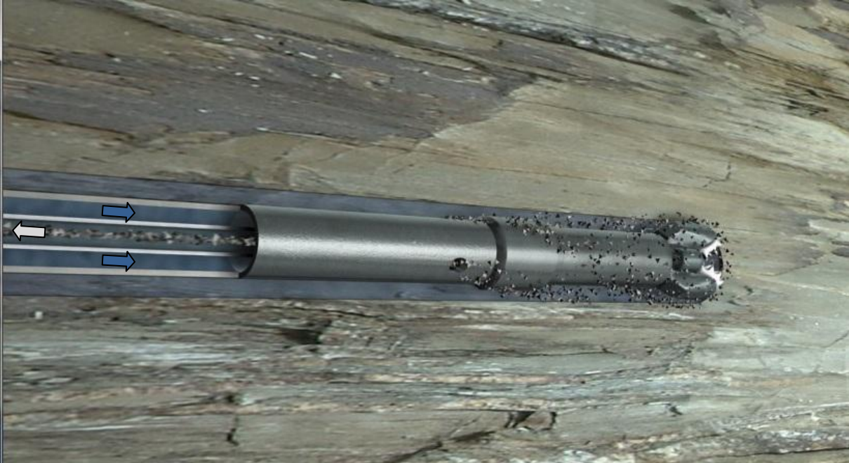
Figure 3.9. Cutting transportation trough the inner drill string using the RDM leaving no cuttings in the horizontal wellbore. (Illustration: Reelwell)
