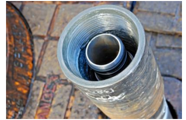
Figure 3.5 Dual drill string used in a RDM test run in Canada. (Photo: Reelwell)
