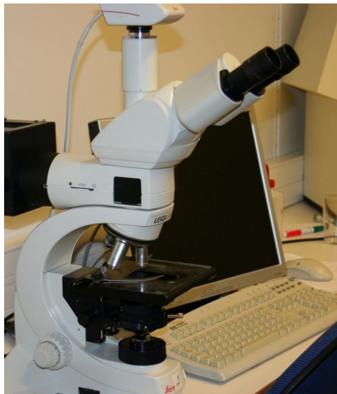
Fig 2.5-2: The Leica DC 100 DMLS microscope with computing software for photographing. Image by Stein-Ove Bratthammer.
