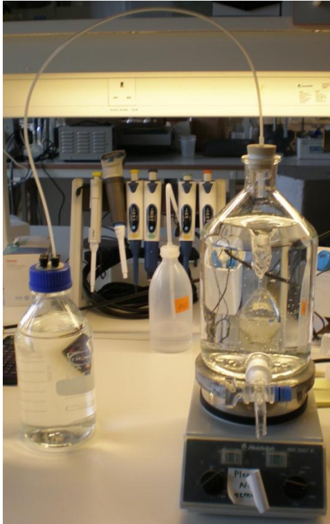
Figure 3-3: Preparation of BTEX test tubes.
