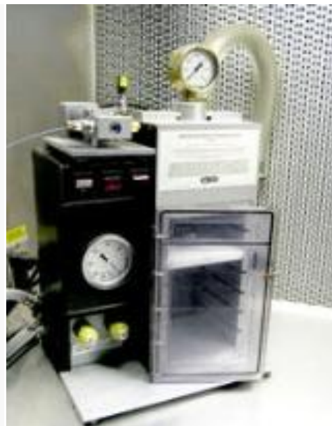
Figure 2.5: The biolistic gun, (Similar to the one used in this thesis) 35
