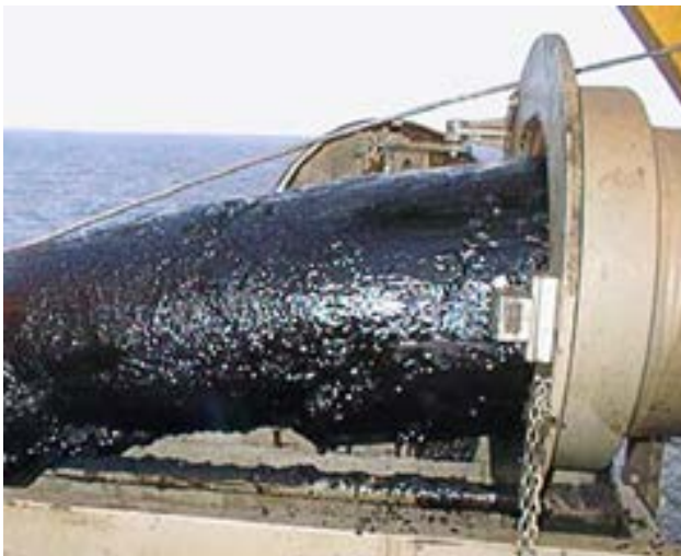
Figure 2 Wax deposition in pipeline (Hydrafact)
