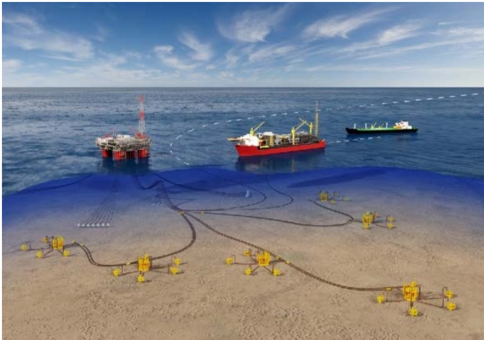
Figure 1 Subsea production system [3].
