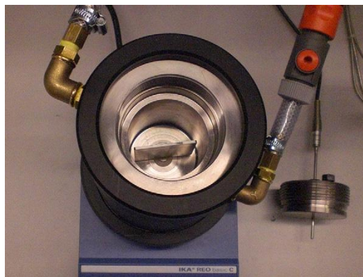
Figure 2.9 Top view of a stainless steel autoclave and screw-top [33].
