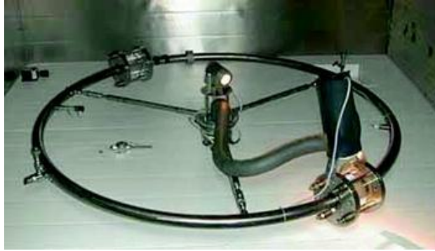
Figure 2.14 A wheel-shaped flowloop (Sintef, Norway) [19].
