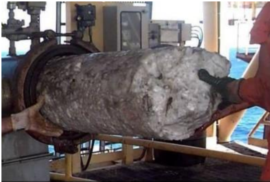
Figure 2.1 Formation of gas hydrate plugged in a subsea pipeline. Picture from Petrobras (Brazil) [19].
