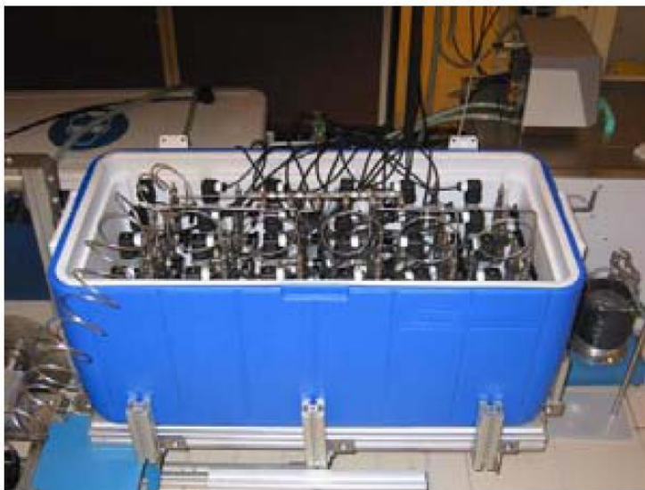
Figure 2.12 Rocking cells used by Shell GSI. The photo at the right shows an individual cell and the main parts, which are comprised by: the 1” tee (1), the end-nuts (2), the pressure transducer (5), a HP quick-connect gas inlet (6), a ball valve (8) and O-ring tightened blind flanges (11). The picture at the left shows the whole cell that contains 24 cells, as it is mounted to the seesaw [35].
