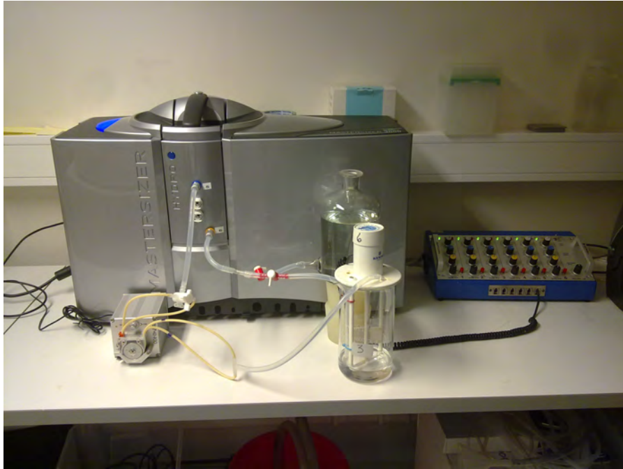
Figure 5.2: Setup for PSD analysis with Malvern Mastersizer 3000 (sampling from flocculation jar test)
