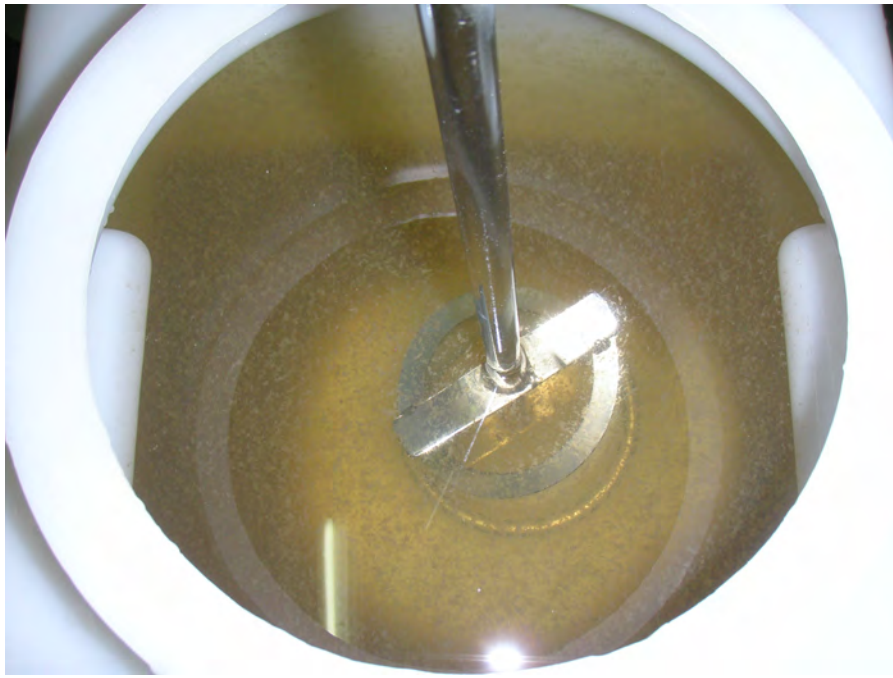
Figure 6.13: Settling of flocs during flocculation with PAX XL-60 and silver stirrer. The settled flocs are visible as a ring around the stirrer and of a darker color compared to the bulk liquid.
