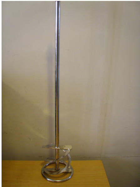
(c) Silver stirrer: Double helix with ring at the bottom. Total length at 300 mm, length of helix at 110 mm and diameter of helix at 100 mm
