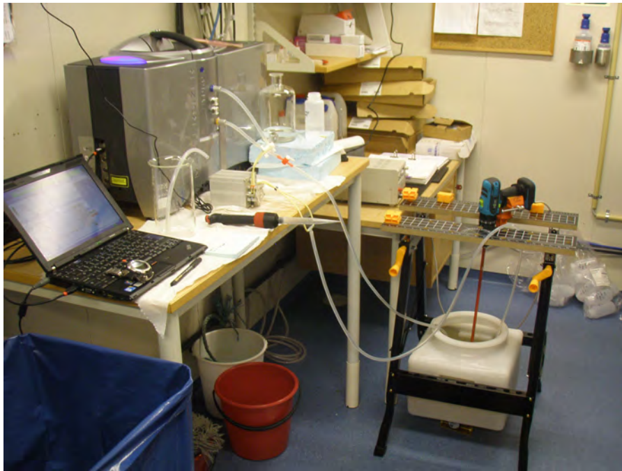
Figure 5.3: Setup for PSD analysis with Malvern Mastersizer 3000 during pilot scale flocculation
