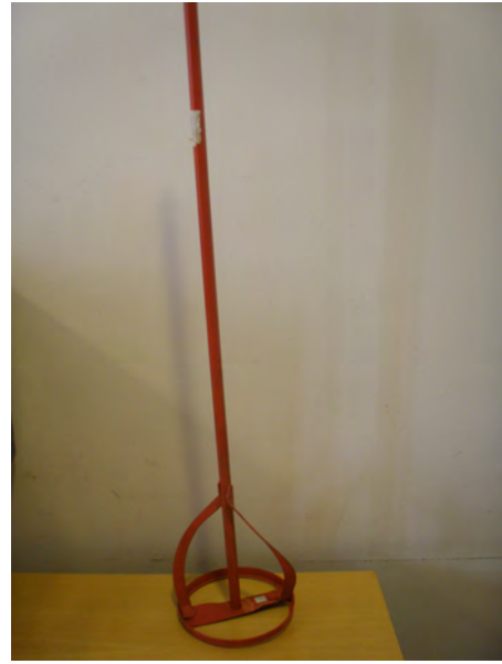
(b) Red stirrer: Double ribbon with ring at the bottom. Total length at 580 mm, length of ribbon at 150 mm and diameter of ring at 115 mm
