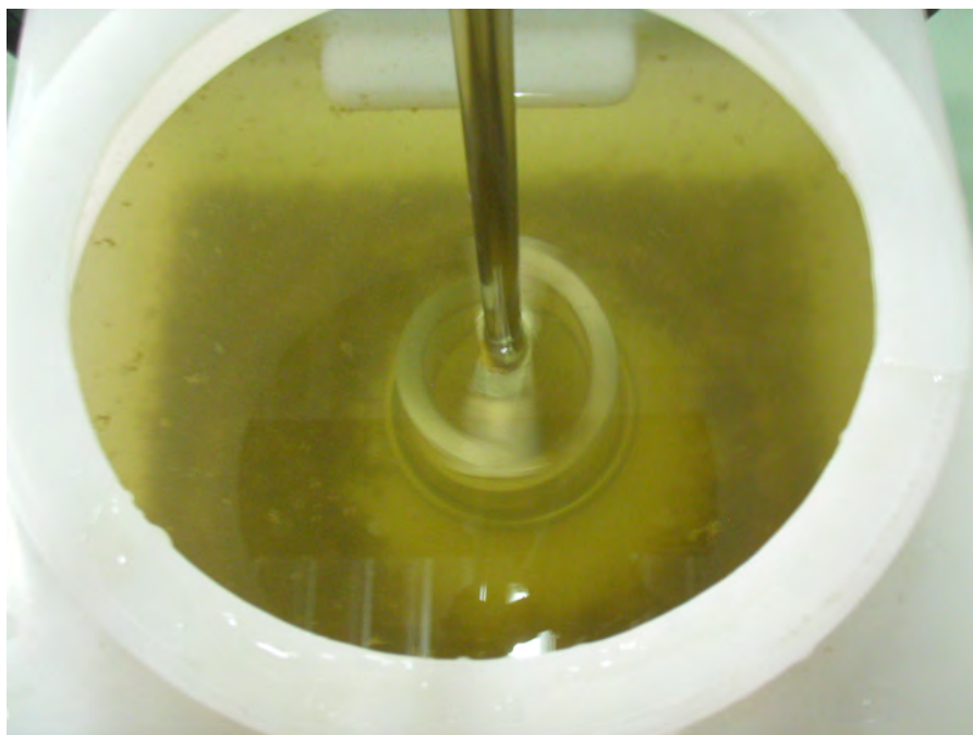
Figure 6.11: Settling of flocs during flocculation with Superfloc C-496 and the silver stirrer. The settled flocs are visible as a ring around the stirrer and of a darker color compared to the bulk liquid.
