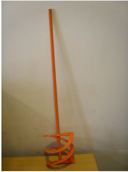
(a) Orange stirrer: Double helix without ring at the bottom. Total length at 590 mm, length of helix at 120 mm and diameter of helix at 120 mm
