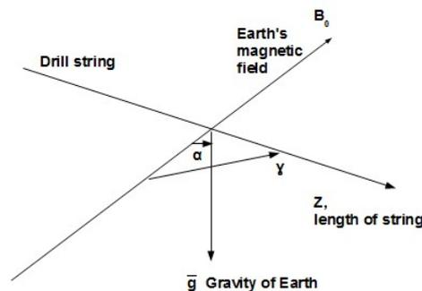
$B_0$  is the magnetic field of Earth. If this drill collar is too short, one can have additional stray magnetic fields influencing the measurements [24]. We want to consider how the pipe's field is influenced by the Earth's magnetic field.  $B_0$ , Earth's magnetic field can be found by measurements.
