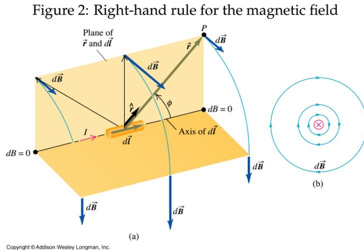
Both equations named **the law of Biot and Savart**. From  $I = n|q|v_d A$  the magnitude of the magnetic field  $d\vec{B}$  at any field point  $P$  is:
