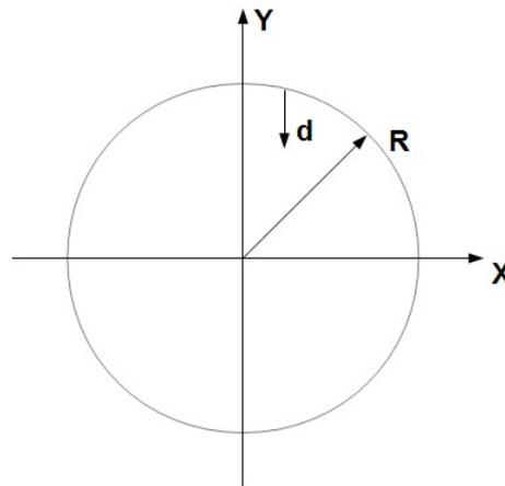
As record in the world the depth of the borehole at 13 km is still "shallow" compared to the Earth's radius of 6384 km. In the non-magnetic drill collar housing the magnetic sensors only have a finite length, and are connected to the steel drill pipe and the bottom hole assembly, with poorly specified magnetic properties. Therefore we don't need to take into account how the Earth's magnetic field changes when the borehole becomes deeper.
