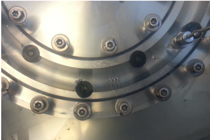
Figure 2.19. A section of the wheel showing the five stainless steel balls added in an effort to increase the turbulence in the system.
