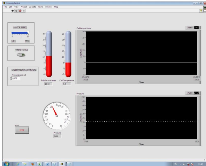
Figure 2.11. The final software interface. Top left is the bar to control the step motor velocity, underneath is the record button for data sampling, then there is a calibration parameter for the pressure and at the bottom a stop button. To the right of this there are two bars, the one to the left is the water heater/cooler temperature and the one to the right is the wheel temperature. Below is the pressure depicted by the pressure meter and by numbers. To the top right is a graphical representation of the wheel temperature, and below is a graphical representation of the pressure.
