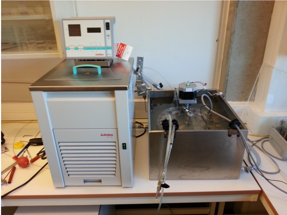
Figure 2.9. The whole assembly with the water heater/cooler to the left and the wheel submerged in the water bath to the right.
