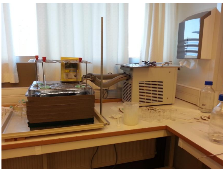
Figure B.1. The THF rig with the water bath together with the rack to hold both the glass rods and beakers on top of it. In addition the thermostat was also there. All this to the left. To the right is the water heater/cooler.
