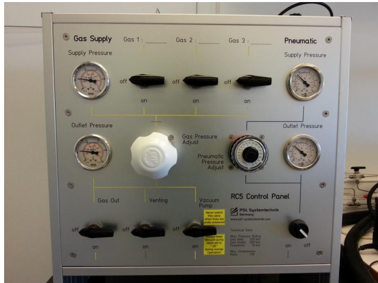
Figure 2.17. The pressure gauge used before the pressure gauge on the wheel had been calibrated. The bottom left pressure gauge was used.
