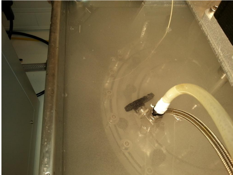
Figure 2.20. The air bubbles severely obstructed the visibility to the wheel making it difficult to observe for hydrate formation.
