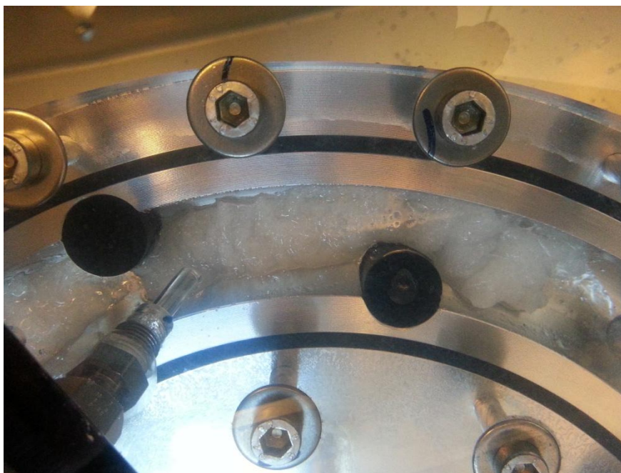
Figure 2.14. A section of the wheel with massive hydrate formation, resulting in a plug of rank E.
