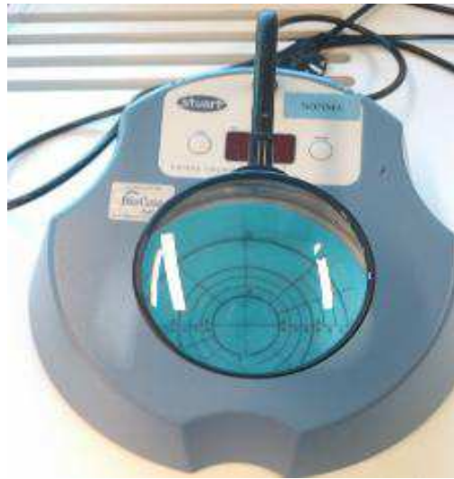
Figure 3.14. a) Counting plate for EDDY JET spreader and colony counts. 3c segment (marked in red) corresponded to the outermost part of a 10 cm Petri dish. b) Colony counter.
