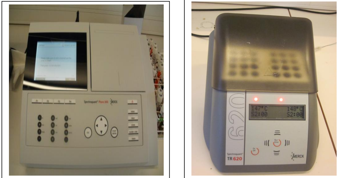
Figure 3.4: Spectroquant Pharo 300 - (left) and Merck Spectroquant thermoreactor (Model TR620) - (right)
