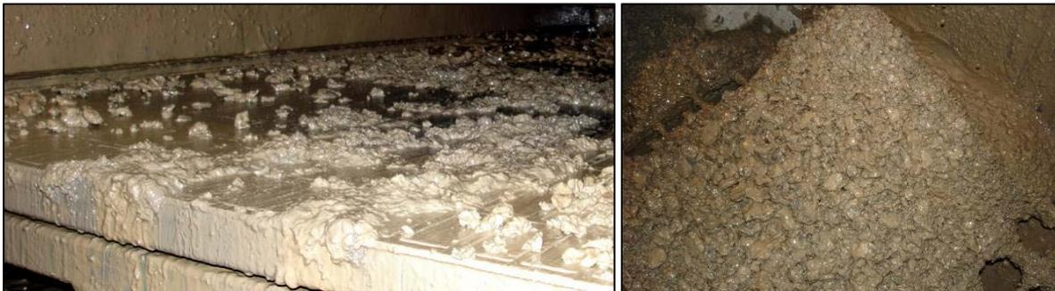
Figure 2-1: Oil based drill cuttings separated from the drilling fluid (Jensen and Halliburton, 2012)
