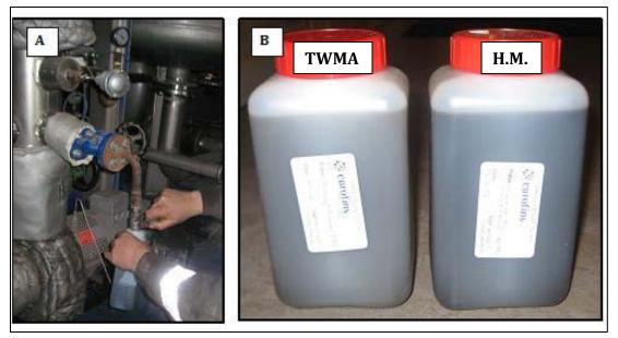
Figure 3-8: A) Sampling of oil B) Visual comparison of oil samples from TWMA and Halliburton Mongstad (H.M.)
