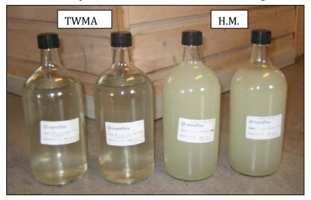
Figure 3-7: Comparison of water samples collected from TWMA and Halliburton Mongstad (H.M.)
