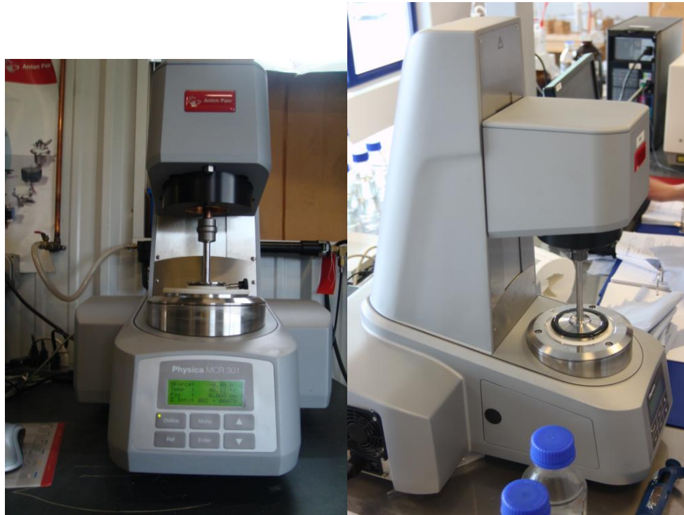
Figure 4-17: A standard Anton Paar rheometer (left) [4] and the rheometer used (right)
