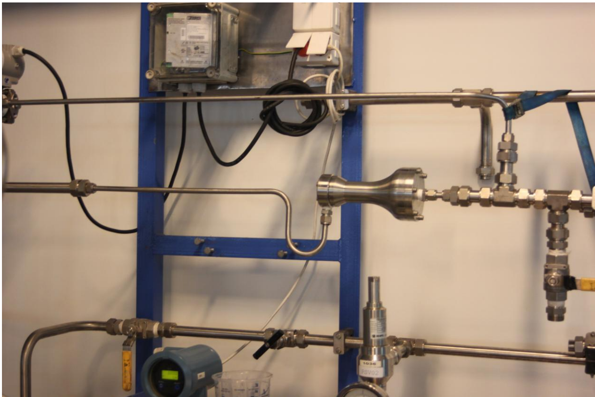
Figure 4-9: The Typhoon valve configuration inserted in the test section of the test-rig
