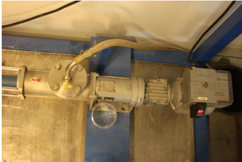
Figure 4-6: The eccentric screw pump used in the test-rig
