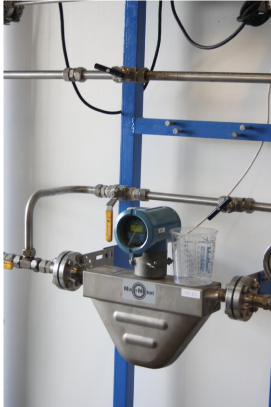
Figure 4-7: The flow meter used in the test-rig
