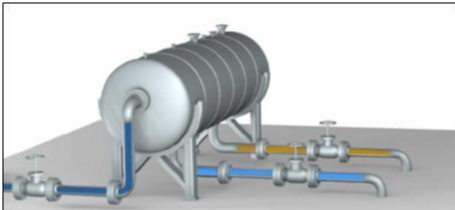
Figure 3-1: Illustration of petroleum processing, the produced fluids are separated into clean phases
