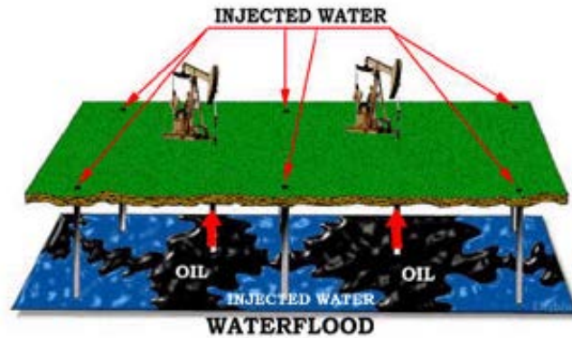
Figure 2.2: The Concept of Waterflooding [Courtesy of Maveric Energy]
