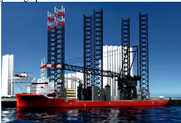
Figure 10 Windfarm Installation Vessel (WIV) [6]
