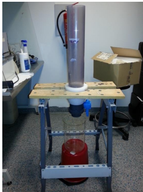
Figure 9. Bench Scale Salsnes Filter setup
