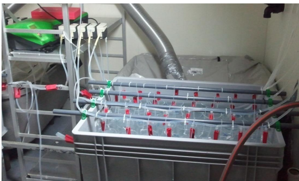
Figure 2.2 General view of experimental setup; header tank, exposure tank and pump.
