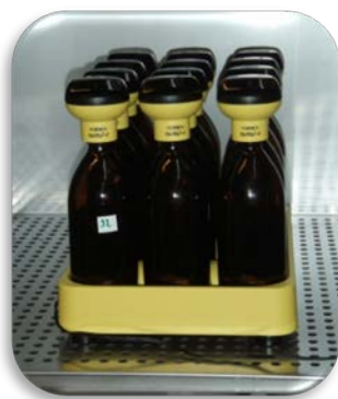
Figure 2.2-1 Test flasks capped with OxiTop®-C heads on magnetic stir plate inside the temperature controlled cabinet.
