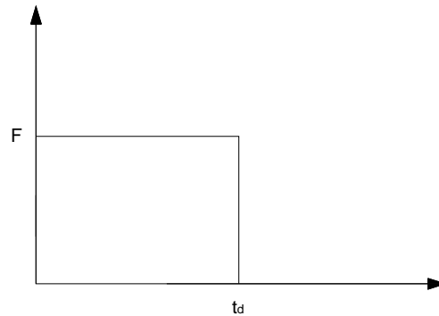
Figure 3.3 Rectangular load pulse (Singelstad, 2008).
