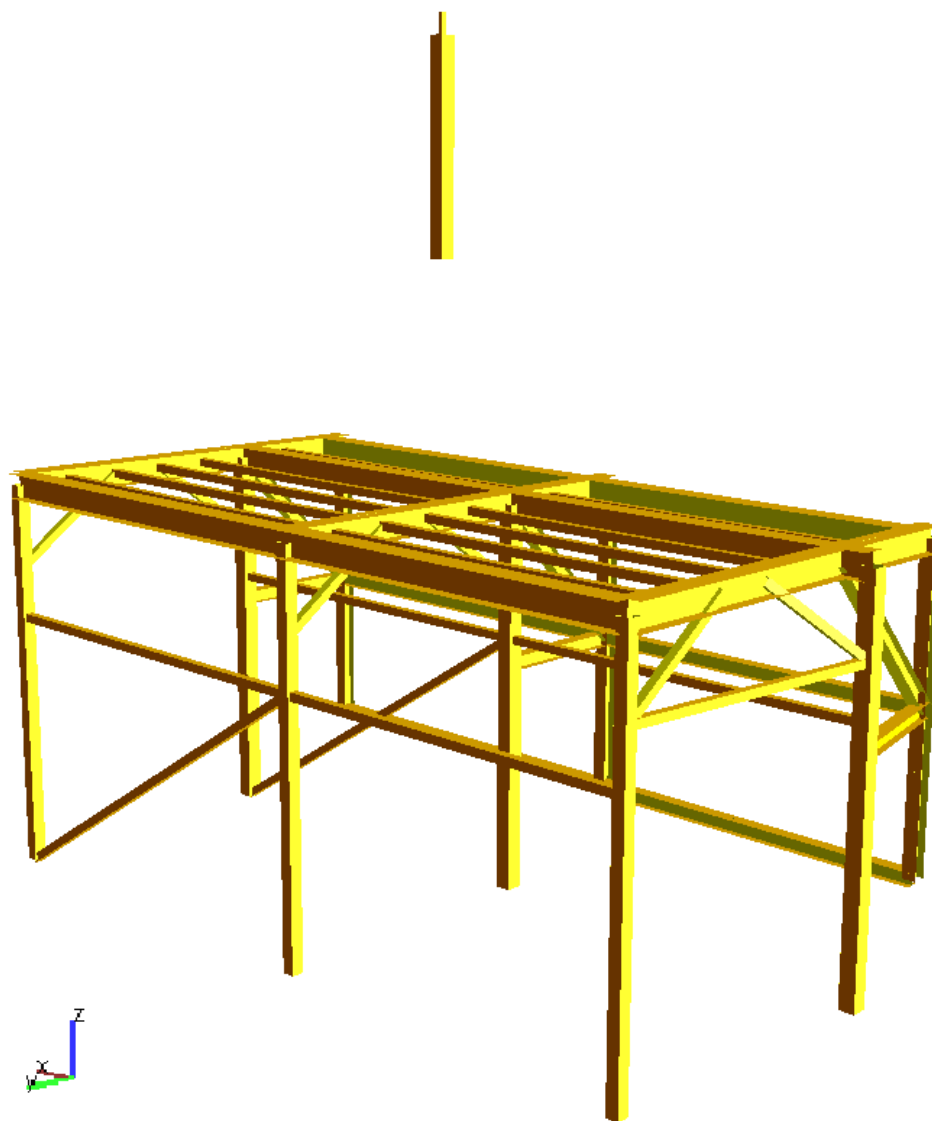
Figure 7.2 Model of laydown area with dropped object (invisible spring).
